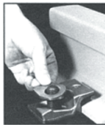
2. Position special washer and lightly tighten nut.
